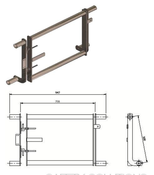
**Evorail Self Closing Gate – ERSWG** Used to safely gain access through the Evorail system. Material – galvanized to BS EN ISO 1461 Compo Component weight – 20 kilos
